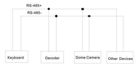
The control system of controlling multiple speed dome cameras is shown as below:
