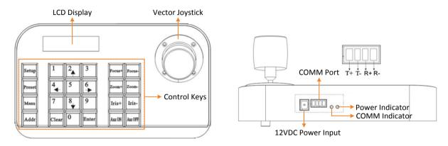
**12VDC Power Input:** Connect to the 12VDC power source.
