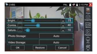
For analog video input, as the resolution is 720\*480, it is normal that the zoom in image is not clear. But for network digital video input, as it supports resolution up to 960\*540, the zoom in image is still very clear. This is very helpful for IP camera installation.
