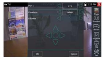
More operation instructions (such as PTZ control, coaxial camera menu setting ,snapshot, recording and playback etc), please refer to "3.3.9 CVI camera test"
