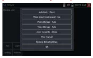
Auto Login: After open this function, tester can auto login camera and display camera image (The login password is the same with last time, the first time using password is the default password "admin")
