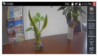
Select relative function on the right side Toolbar to operate, functions including "Photos", "Snapshot",
