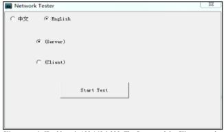
Tester as Client, tester's IP address is:192.168.0.238. The Server and the Client are at the same network segment, but with different IP address. Input Server's IP address 192.168.0.237 in the tester and click "Start" to test network bandwidth.
