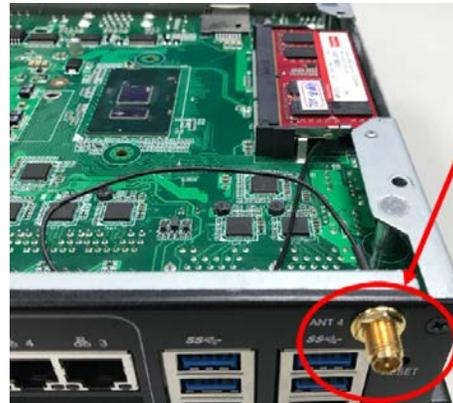
4. Screw the GPS antenna to the Antenna port.
